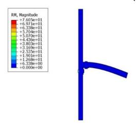
Figure 6- Bending moment distribution in wood structure (N/mm)
