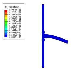
Figure 4- Bending moment distribution in wood structure in N/mm
