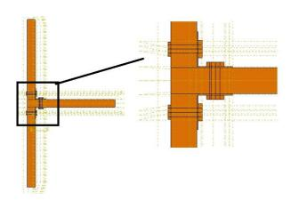
Figure 1- Schematic of finite elements model and elite, bolt and nut joints on one side
