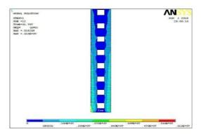
Figure 11: stress contour of the lower wall in the unretrofitted model
