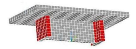
Figure 1: The FRP-reinforced wall of Kheyroddin
