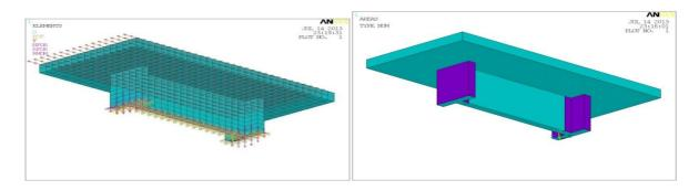
Figure 2: Elements used formodelling, meshingand loading the wall
