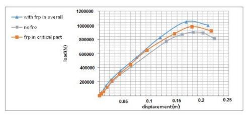
Figure 25: Comparative diagram (load-displacement) of walls with and without FRP
