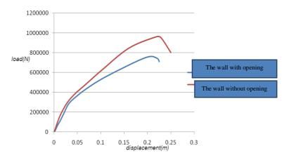
Figure 17: comparison of the pushover curve for the wall with and without opening
