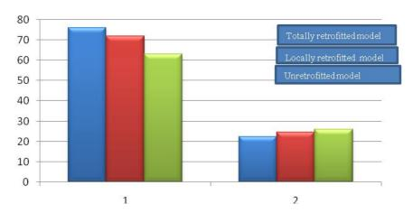
Figure 13: comparison of bearing capacity and ultimate displacement of the models, 4, 5 and 6
