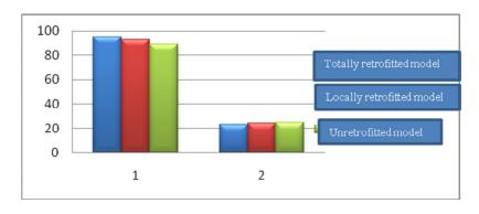
Figure 9: Comparison of bearing capacity and ultimate displacement of the models 1, 2, 3
