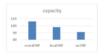
Figure 26: Capacities of walls for three models
