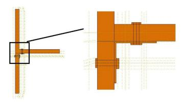
Figure 1- Schematic of finite elements model and elite, bolt and nut joints on one side
