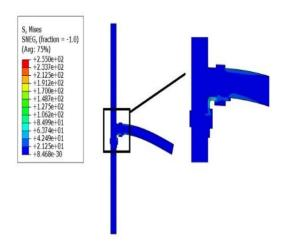
Figure 5- Tension distribution in wood structure (Mpa)
