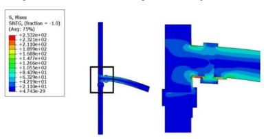
Figure 3- Tension distribution in wood structure (in Mpa)
