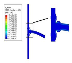
Figure 5- Tension distribution in wood structure (in Mpa)
