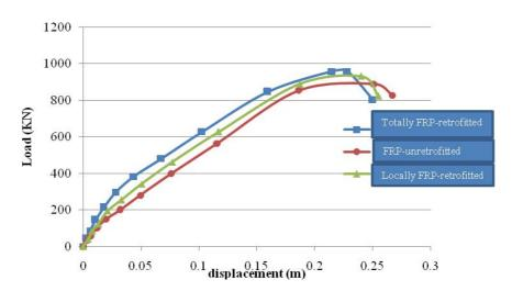
Figure 8: Load-displacement curve for the models 1, 2, 3
