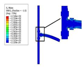
Figure 3- Tension distribution in wood structure in Mpa
