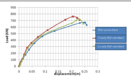
Figure 12: load-displacement curve for Model 4, 5 and 6
