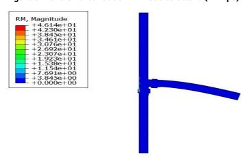
Figure 4- Bending moment distribution in wood structure (in N/mm)
