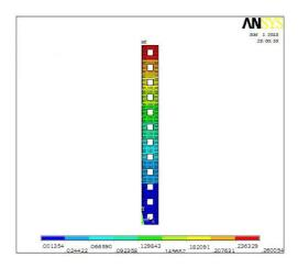
Figure 10: horizontal displacement of the Model 4
