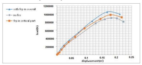
Figure 20: Comparative diagram (load-displacement) of walls with and without FRP
