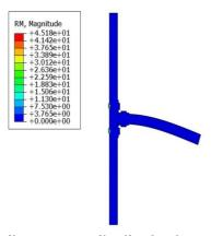
Figure 6- Bending moment distribution in wood structure
