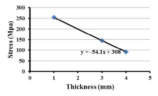
Figure 7- The changes of tension distribution with the increase of thickness of elit
